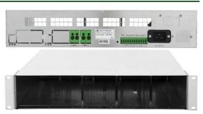
The LS1500 type power sources are designed to back up supply devices and to simultaneously charge the connected battery. In case of mains failure the connected battery continues to supply load without interruption. The power source unit is designed as a plug-in module that can be added or replaced during operation, without a need to turn the system off.
