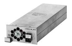
The LS300.Z 48\_2415 DC converter is a plug-in unit for LS1500 chassis. DC/DC converter is built in most advanced technology with of the energy conversion with respect to maximum efficiency (ZVS). The unit provides 24V adjustable output up to 420W. Soft start, temperature controlled fan switching, input and output filter are some of the main features.
