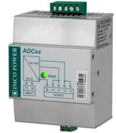
DC/DC converters type ADC01.H convert 48V DC input voltage to 24V DC output voltage. Output is galvanically isolated from the input, output terminals are doubled. The LED on the front panel indicates the presence of the output voltage.
