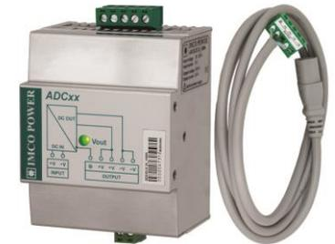
DC/DC converters type ADC02.H with 24V (48V) DC input voltage are designed to supply devices with input voltage 100-230V~50/60Hz up to 100W without needs a DC/AC inverter. For this purpose, a part of the delivery is a special cable for supplying of this device. Output is galvanically isolated from the input. The LED on the front panel indicates the presence of the output voltage.
