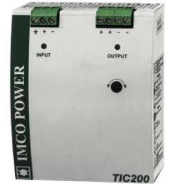
The TIC200.H DC/DC converters convert 24V (48V) input voltage to 12V (24V, 48V, 220V) output voltage with galvanic separation. DC/DC converters are equipped with a local LED indication located on the front panel. There is possibility of output voltage trimming (see specification table).
