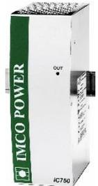
The power supply type IC750.H 22003 is intended for to supply devices with 220VDC input voltage and up to 660W. The IC750 allows long life operation in industrial environments from -25°C up to +50°C ambient temperature. Class D surge protection, short-circuit protection and galvanically isolated output are some of main features of the power supply IC750.H 22003 types additionally have an output with IU voltage characteristic.
